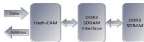
Fig2:Hash-CAM lookup circuit using DDR3 SDRAMs
